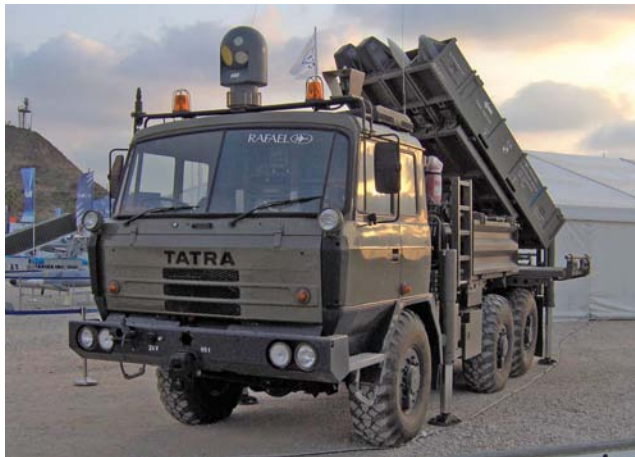
Figure 10. Advanced SAM systems, such as the SPYDER that combines Python-5 EO-IR missiles with active radar-guided missiles, can provide highly capable area defense capabilities. (Reprinted from Wikipedia , s.v. “SPYDER,” accessed 20 June 2011, http://en.wikipedia.org/wiki/SPYDER .)
