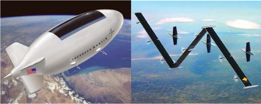
Figure 24. Persistent near-space systems, potentially in the form of ultra-long-endurance airships or autonomous flight vehicles, can ensure theater-level communications relay functions in the event of loss or degradation of corresponding space systems. (Courtesy Lockheed Martin [left] and “DARPA’s Vulture: What Goes Up, Needn’t Come Down,” Defense Industry Daily , 16 September 2010, http://www.defenseindustrydaily.com/DARPA-s-Vulture-What-Goes-Up-Neednt-Come-Down-04852 [right].)
