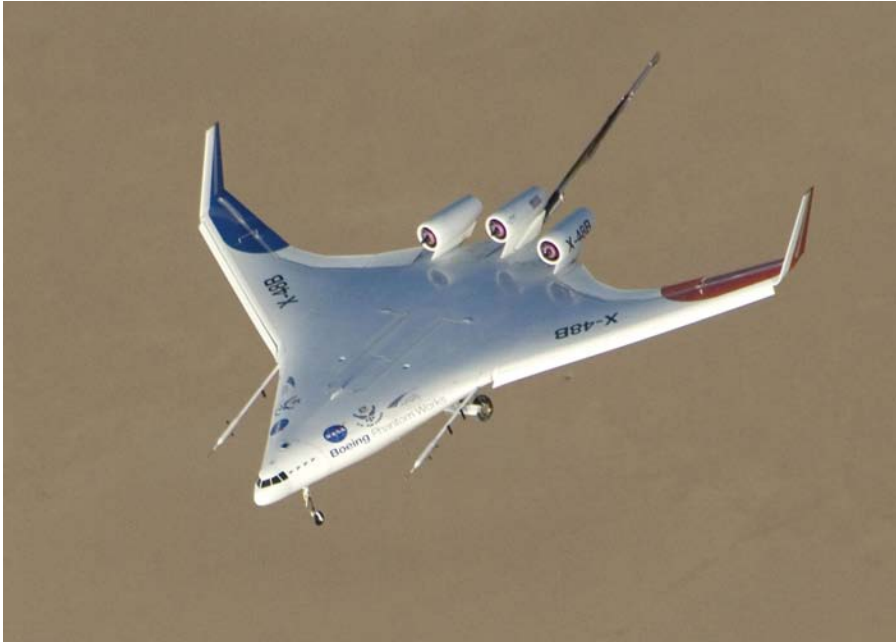
Figure 28. Hybrid wing-body aircraft have higher fuel efficiency than traditional tube-and-wing designs for tankers and transports. Advances in integrated stitched-composite manufacturing technologies such as PRSEUS (pultruded, rod-stitched efficient unitized structure) have enabled large, lightweight, high-stiffness panels at low cost. (Courtesy NASA/Dryden.)
