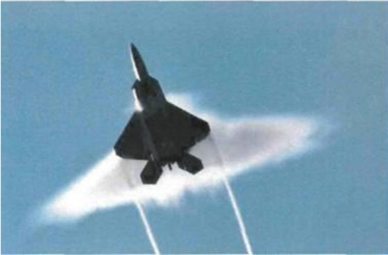
A U.S. Air Force F-22 'Raptor' executes a supersonic flyby at low altitude, producing pronounced wingtip vortices and a 'shock egg'.
