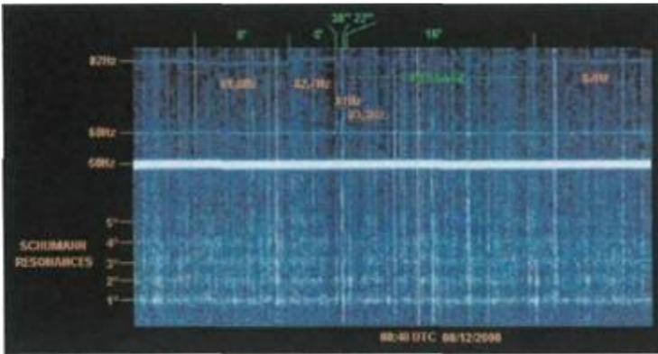
A ZEVS transmission recorded in Italia by Renato Romero on the 8th of December 2000, at 08:40 UTC. The "message waiting" signal, 81.6 Hz low for 8 minutes, 82.7 Hz high for 4 minutes is easily detected in the spectrogram. After the 16 minutes long message sequence of the transmission is again the carrier at 82 Hz. Because of the long exposure are the Schumann resonance bands easily visible at the bottom of the spectrogram.
